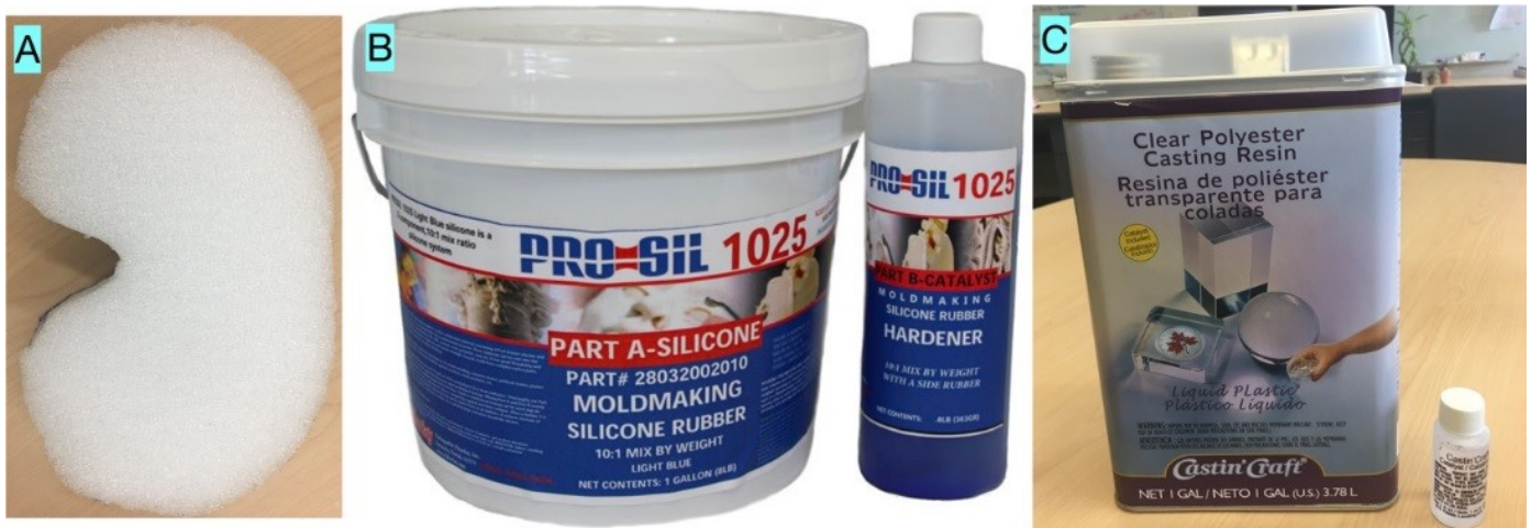
Figure 9. Essential materials used to cast the anthropomorphic phantom. A – Foamboard; B - Prosil Silicone RTV Mold: left - silicone rubber; right - hardener C - Castin' Craft Clear Polyester Casting Resin: left - resin; right – catalyst.
